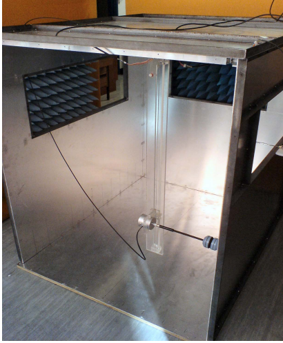
Fig. 2 Simple rectangular cavity used for field measurements at 870 MHz and 1800 MHz
